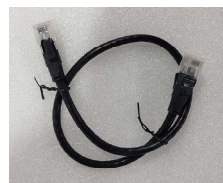
Communication Connection Line RJ45 for RS485/CAN
