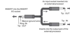
The output signal of the INSERT socket is reversed. This should not be m M a problem when connecting to effects units, but be aware that there may be phase conflicts when connecting to other types of devices.
